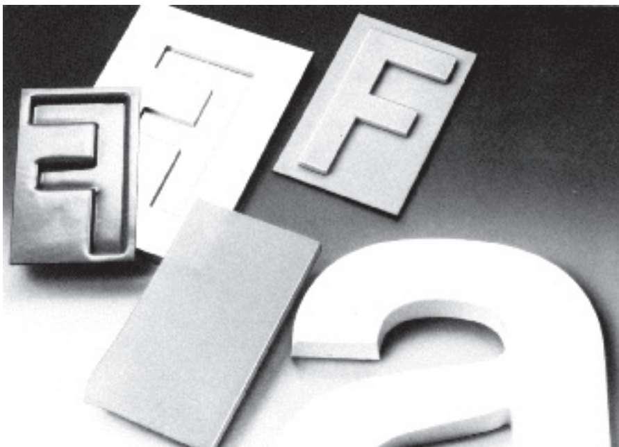
Fig. 20: PLEXIGLAS® GS letters pressure-formed using an aluminum mold and silicone rubber sheet
